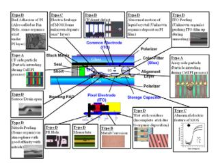
Figure 2. Classification of defect of TFT/LCD panel.
