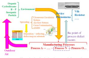
Figure 7. Hypothesis of relation between defect and environment.
