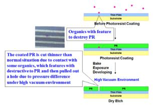
Figure 2. Mechanism of formation of overetched defect.
